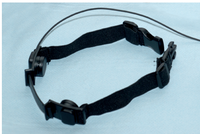
Figure 1. Contact microphone (CTH100, Clockaudio Ltd., Waterlooville, UK), utilized for high signal-to-noise ratio clinical recordings of snoring audio data.
